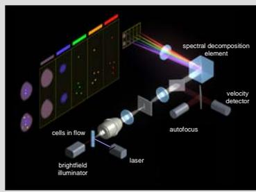
Fig. 1. Schematic representation of the Imagestream® 100
